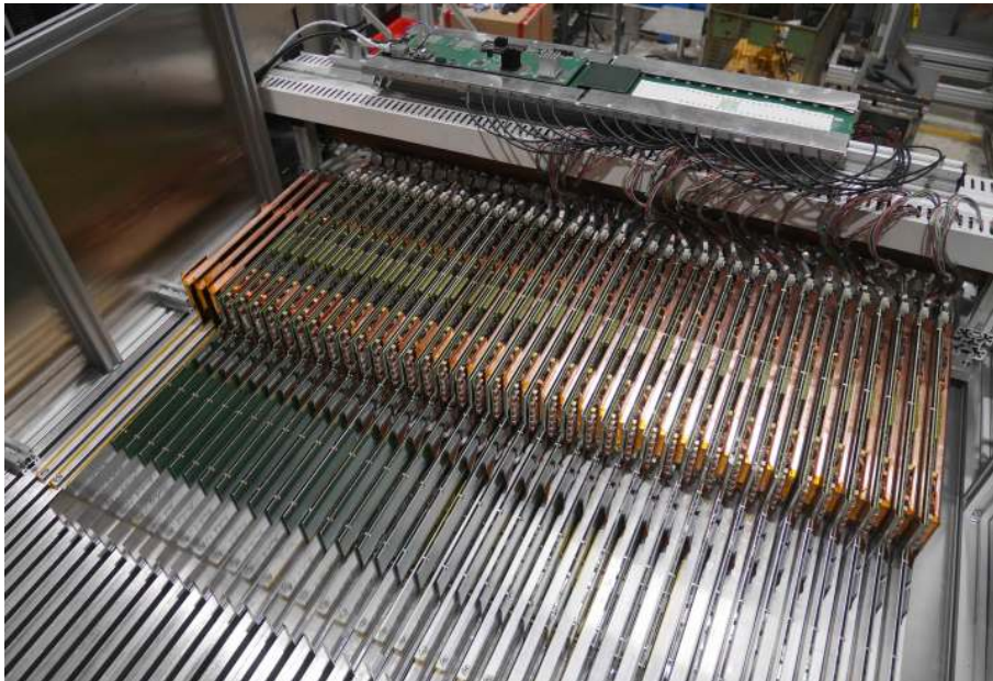
Figure 4.4: View on the top of the (opened) 2018 AHCAL engineering prototype fully assembled with 38 active layers. The picture was taken during test beam at SPS in May 2018.
