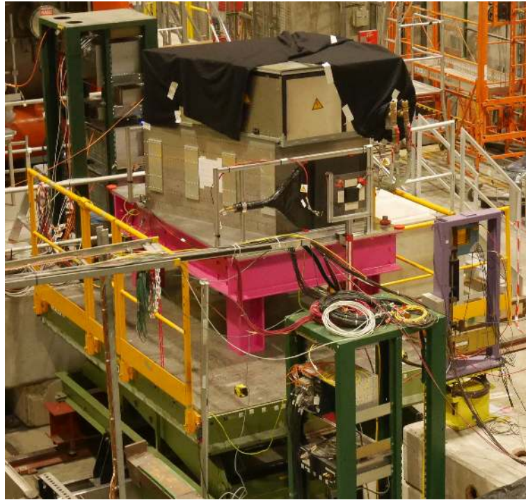
Figure 4.6: May 2018 test beam setup at SPS north area, beam line H2. The covered AHCAL prototype on a movable stage with DAQ system and cooling behind the detector. Beam incident is in the front of the detector from this point of view.
