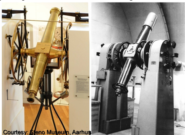
Figure 2 Left: the Copenhagen meridian circle as used in 1925 – by Pistor & Martins, Berlin, 1859. Right: the new meridian circle by Grubb Parsons, Newcastle, installed in 1953 at Brorfelde, 50 km to the west of Copenhagen. – EH
