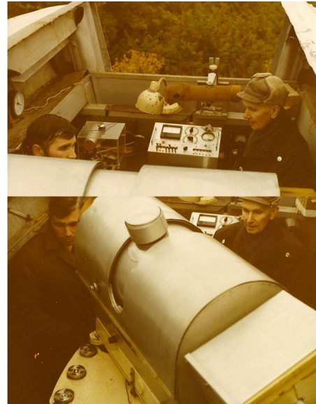
Figure 5 Pulkovo Observatory in 1978. N.N. Pavlov at right pioneered photoelectric astrometry for time service with a transit instrument, G.I. Pinigin at left. The instrument is reversible as seen in the lower part of the figure. - EH
