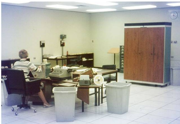
Figure 15 Computer room of Perth Observatory 1971. GIER in the brown cupboard was one of the first transistorized computers. Mrs Ilse Holst at the reader for 8-channel punched tape, one role could contain 0.00012 Gbytes. The tape from reader or punch poured into a large basket and could then be quickly rolled up. - BL
