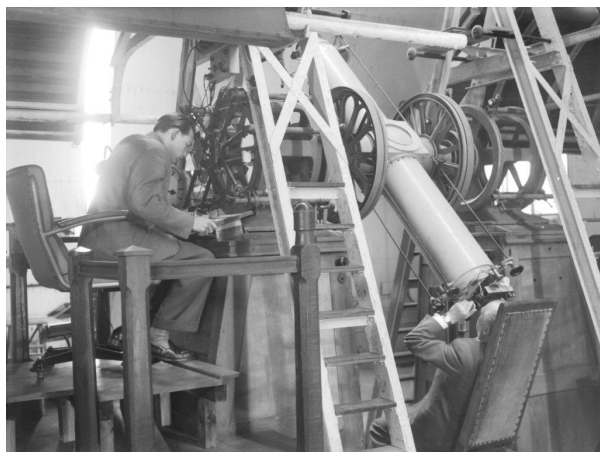
Figure 8 The Repsold meridian circle about 1960. Gerhard Holst is reading the declination circle and Johann von der Heide is observing the star with the visual micrometer. - WD
