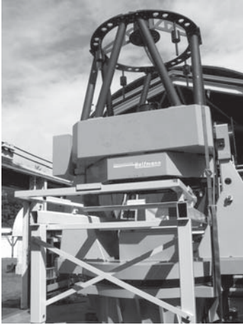
Figure 19. STELLA (STELLar Activity), the new 1.2m robotic telescope to be operated on Tenerife to study stellar activity. Hamburger Sternwarte.
