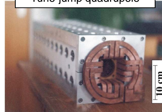
Panofsky-type quadrupole with ferrite yoke
