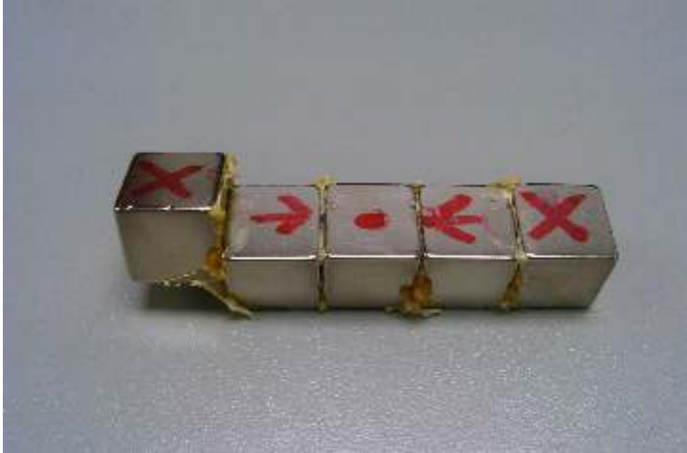
Figure 5.15.: A 5x1 array with one of the outermost magnets out-of-band. This is a result of too much glue applied between this magnet and the neighbouring one. It can also occur if too less glue is used or, regardless of the amount of glue, if there are external forces exerted on the outermost magnet after the array is detached and stored.
