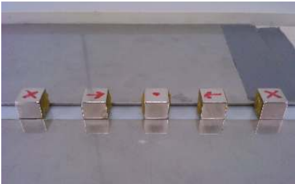
Figure 5.10.: Magnets placed inside the rail with glue put on the inner faces. The marks on the upper faces indicate the direction of magnetization; the arrows point towards the south pole which is indicated by the dot. The cross indicates the north pole. This is in analogy to the sketches in figures 4.3 to 4.5
