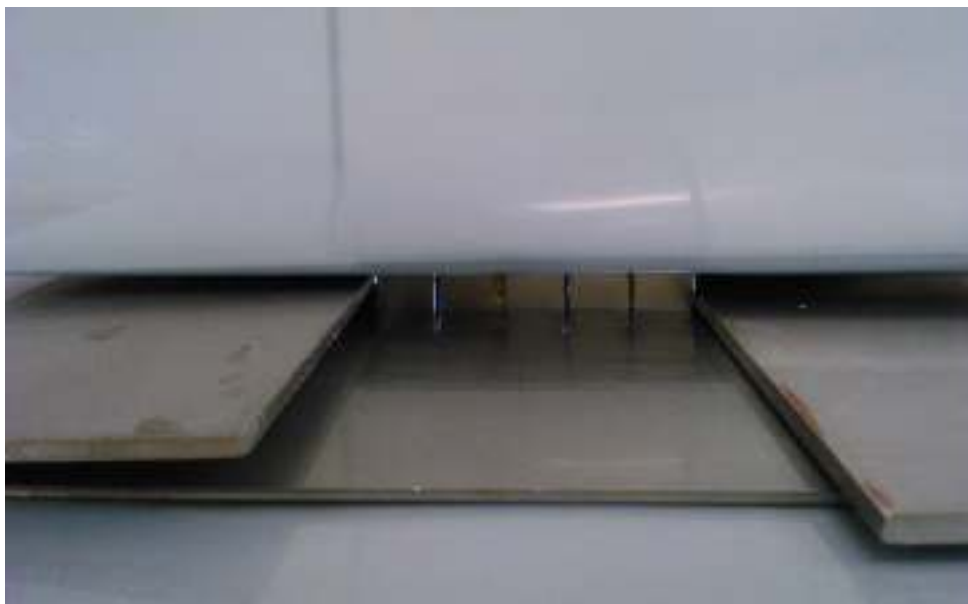
(b) magnets in rail after being pushed together
