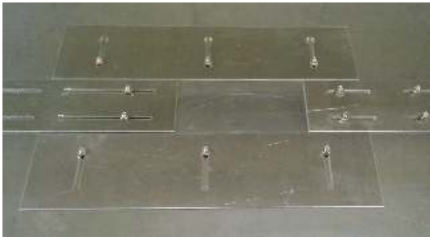
Figure 5.21.: The new rail for the glueing process. Again, the basis is an iron plate. The four aluminium plates with the long holes can be moved in one direction each. Once they are positioned correctly, they can be fixed via the screws and the nuts. In a first step the “upper” plate (related to the figure) and the one on the right side are fixed. After the stripes are put onto the iron plate and brought into line with the edges, the “lower” plate is moved towards them and then also fixed. This way, the stripes are bound in three directions. The plate on the left side can then be used to push them together and, after also being fixed, bound them in the remaining direction.
