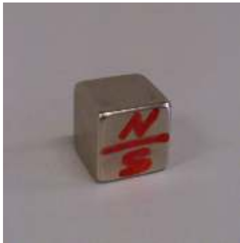
Figure 5.1.: A single cubic magnet used for the preliminary measurements for BRASS. The magnetization direction lies parallel to the centre line between the upper and the lower faces in this picture.
