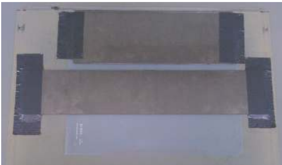
Figure 5.9.: The fully prepared rail used for the fixation of the magnets while glueing them together. Its components are described above.
