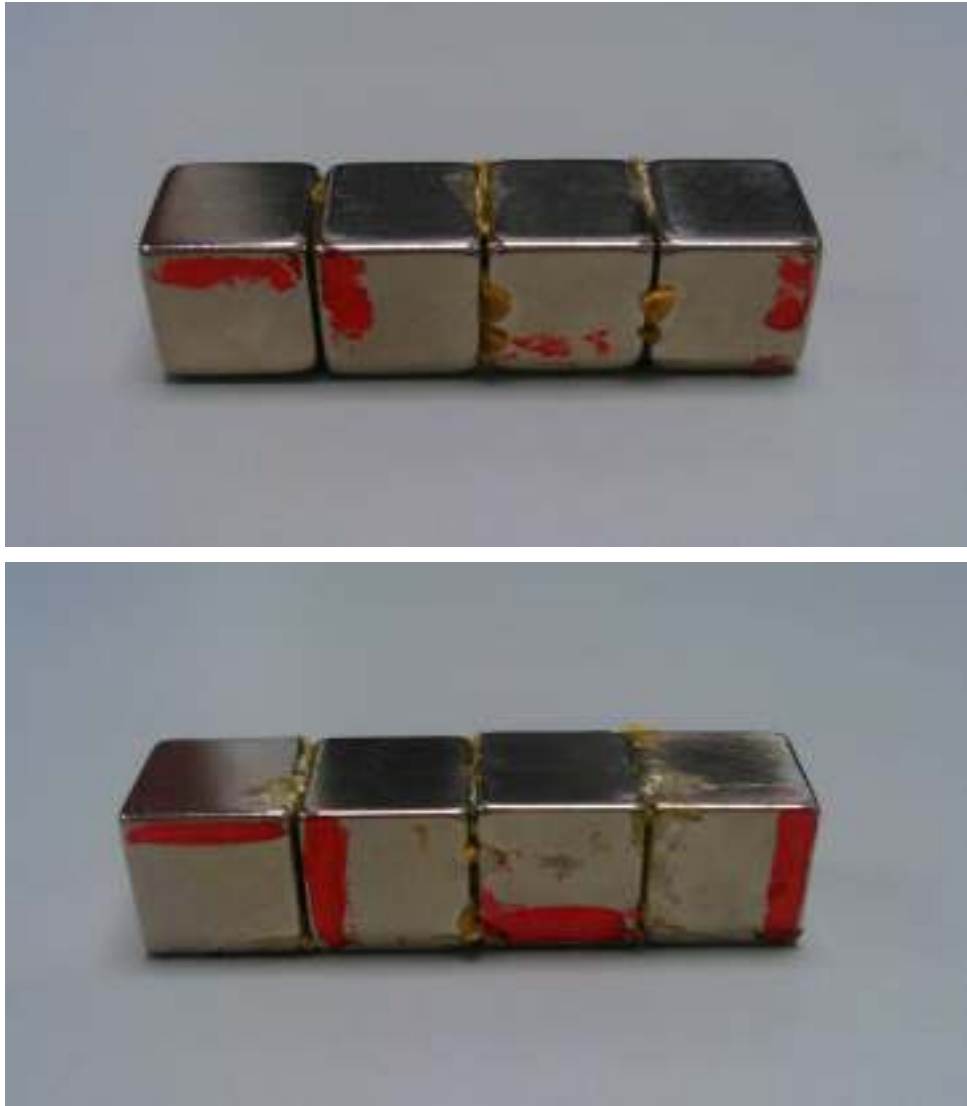
Figure 5.16.: The 2 constructed 1D Halbach units. The red bars indicate the south poles of the magnets. It is clearly visible that there is some space between the individual magnets due to the glue. The unit is therefore slightly wider than the sum of the 4 magnets. In the middle of the lower unit it is also visible that the arrangement is not perfectly planar. This also applies to the upper unit, though it is harder to see in this image.
