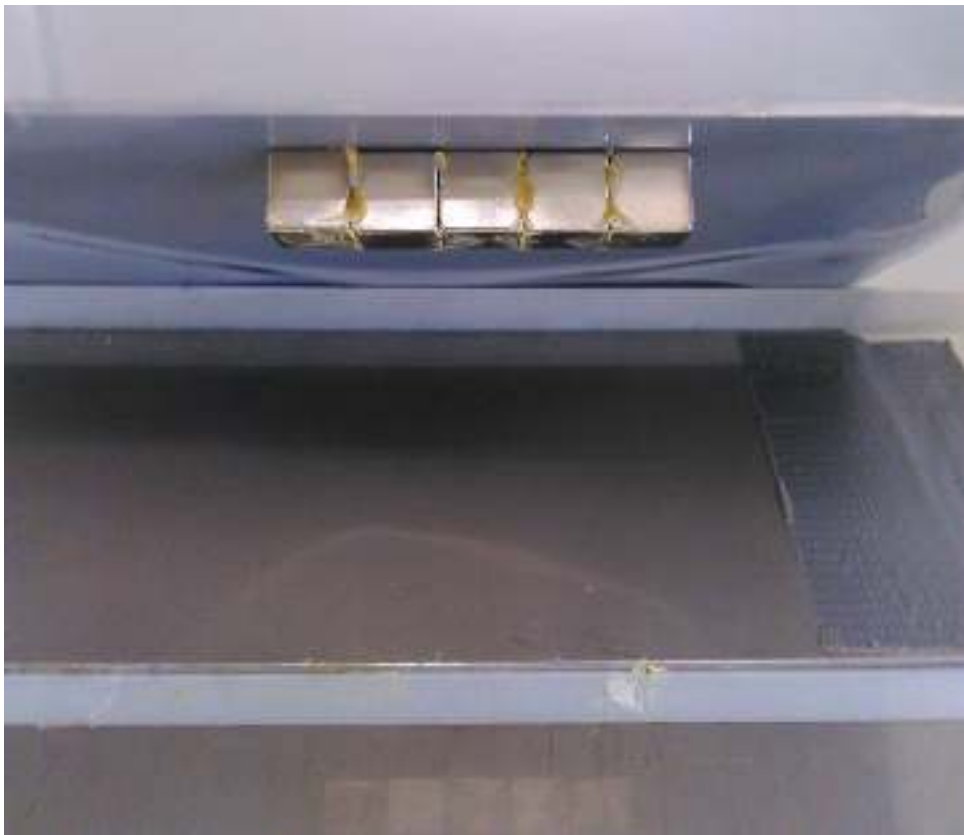
Figure 5.12.: The glued magnets from figure 5.11(b) after detaching them after the glue hardened. Since the magnetic field is stronger on the upper side, the array sticks to the upper plate. This plate is smaller and it is therefore easier to release the array afterwards from this one than from the bigger lower plate.
