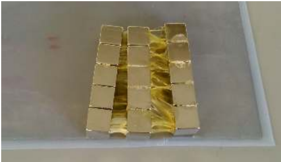
Figure 5.23.: The result of the first failed attempt. These three stripes could be pushed together, but it was not possible to push them further towards the remaining two stripes. Although still attracted by the small iron plate, they moved a little bit away from each other due to their repellent forces. This is indicated by the glue between them: to end up in this state, the inner surfaces must have been so close that the glue drops applied to them were in contact with each other. Apparently, the glue was insufficiently strong to hold the magnets together and was elongated instead.
