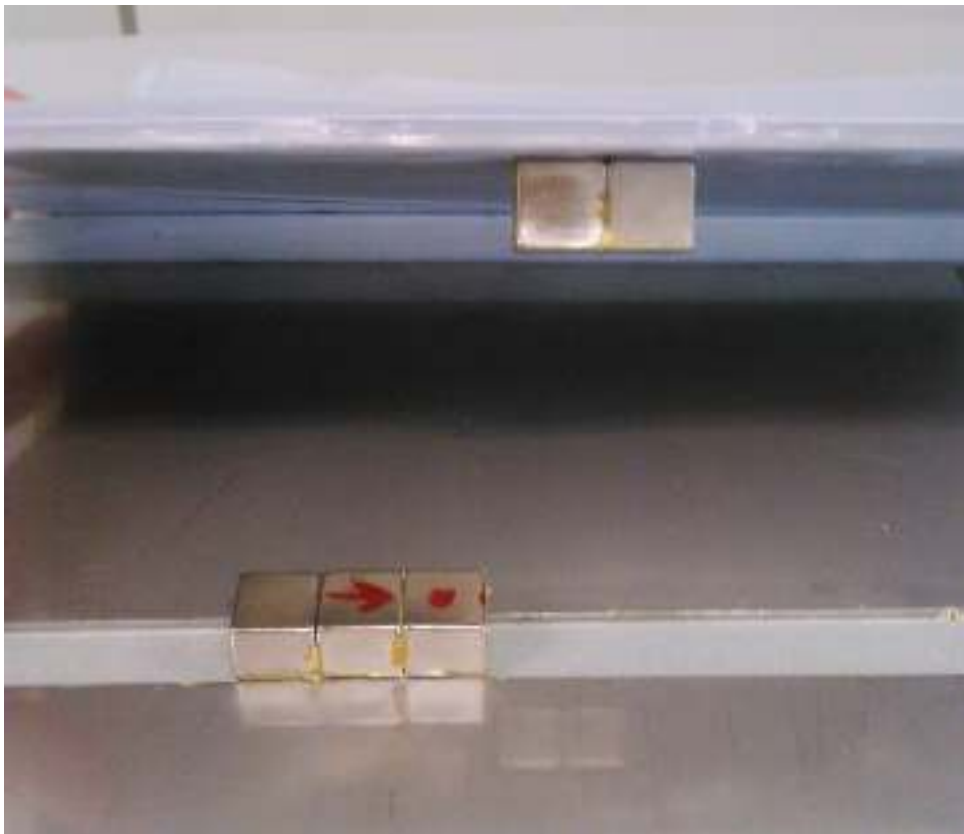
Figure 5.14.: A 5x1 array damaged while being detached from the lower plate. As a result of glue seeping between the three magnets on the left and the lower plate, their attraction was stronger than the adhesive attraction between the three magnets on the left and the two magnets on the right. Hence, the attempt to detach the array resulted in the breaking of the array.
