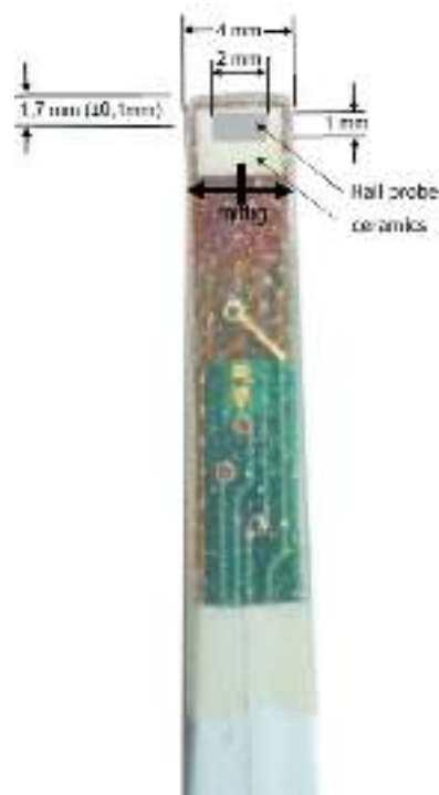
Figure 5.3.: A sketch of the Hall probe used for the magnetic field measurements. The tip of the probe contains the active area, which is surrounded by ceramics. This area has the size 1\text{ mm} \times 2\text{ mm} and its middle is 1.7\text{ mm} inside the tip.
