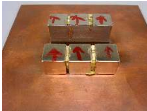
Figure 5.20.: Setup of different preliminary measurements for BRASS. The magnets were glued together as described in section 5.3. Due to the normal force between the magnets, the glue was stretched while hardening. The array is therefore stable but includes measurably large gaps between the magnets. See [52] for further detail.
